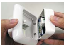
Figure 3 Holding two side of body, to take body off base part
