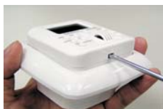
Figure 1 Using screw-driver push hook backward
